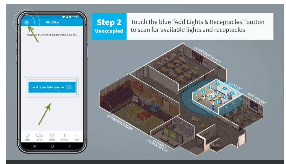
The "Add Lights" section offers two ways to add lights. Touch the blue "Add Lights & Receptacles" button or the plus "+" symbol to scan for available lights within range.
