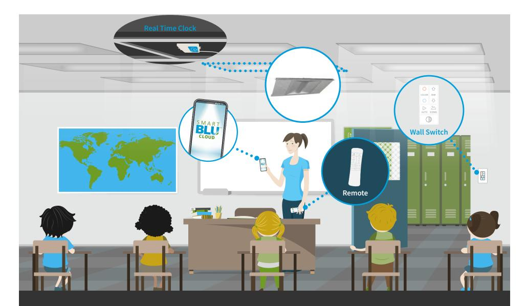
A light network is a wireless association of light fixtures embedded with motion/photo sensors and control devices such as wall switches, remotes, and real time clocks. You can have up to 100 lights and devices on one light network but most often it will be much less.
