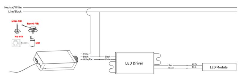
Note that the Line/Black is shared between BBR-RP and the LED Driver. Dimming control occurs via White/Red connecting to LED Driver White.
