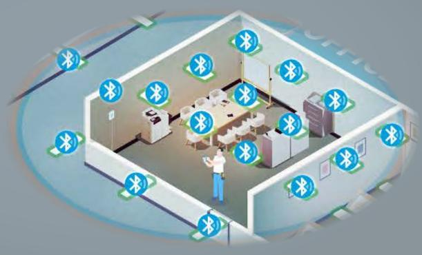
After scanning, SMART BLU<sup>®</sup> will display a count of all lights that were reached on the bottom left corner of the screen. Compare this against the number of lights counted within your area. In this example, the app shows 17 lights whereas there are only 9 lights in the room.
