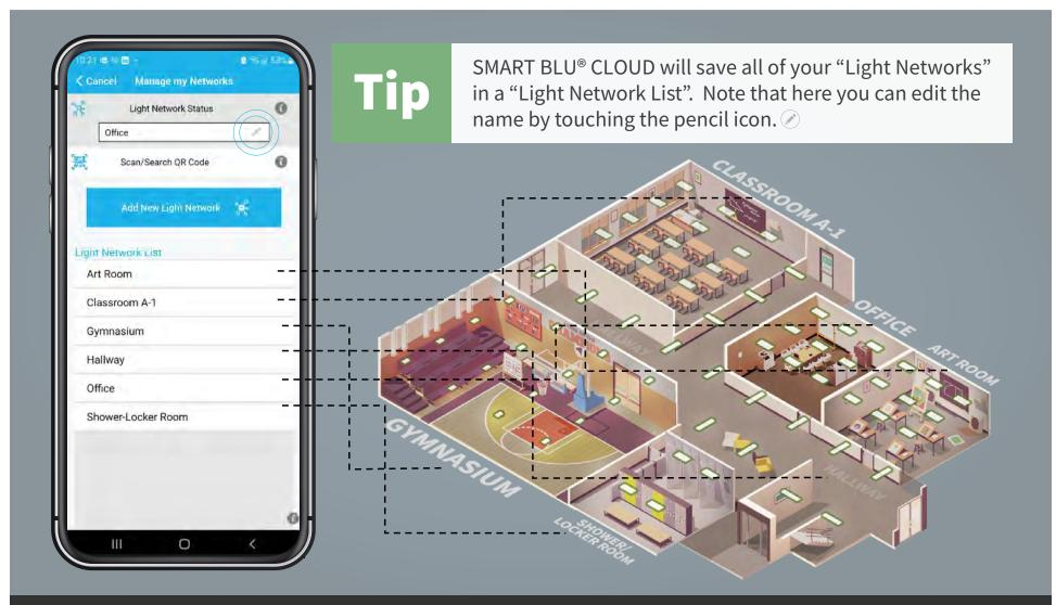
Light Networks created are saved in an easy to navigate list found in the "Manage my Networks" section. Simply touch the name of the Light Network you wish to join and the app will automatically connect. Note that you must be in the space while connecting.
