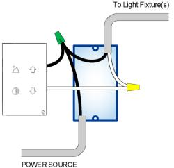
For the SBWS-4B, power is paralleled to both switch and Light Fixture(s). This is because the SBWS-4B™ controls the Light(s) via wireless communication. Power must be continuous to both switch and Light(s).
