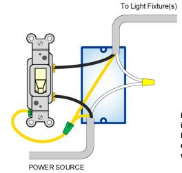
Note that pwer is interrupted going to the Light Fixture(s) in the conventional toggle style wall switch.
